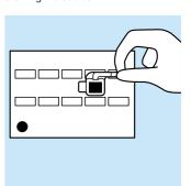
Shake pack well to mix the active chemical ingredient with test solution. Then compare resulting solution color to chart and determine density level.
