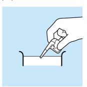
Dip nozzle into test solution. Squeeze pump then slowly release your fingers drawing the solution.
